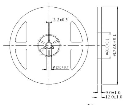
Unit: mm Tolerance:  $\pm 0.25$ mm
