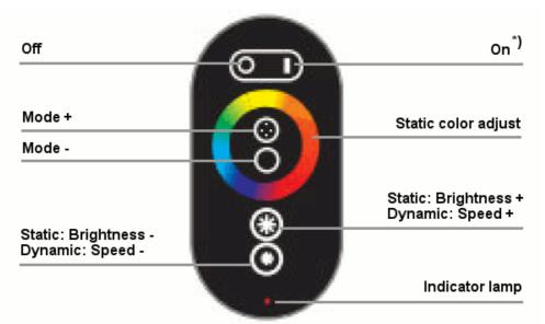
\*) Remote controller is going to sleep mode after 30sec no use and doesn't respond to any sensor touch buttons. Reactivation by pressing the ON button one time at least.
