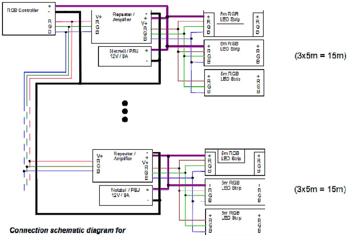
**Connection schematic diagram for Repeater-supported RGB applications**
