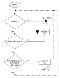
Brightness control, presence detection and automatic switch-on can be activated and deactivated using various modes. Brightness reduction
